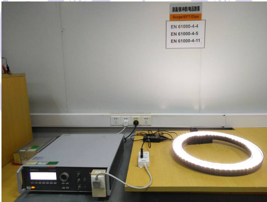
EFT & Surge & Voltage Dips & Voltage Interruption Test View
